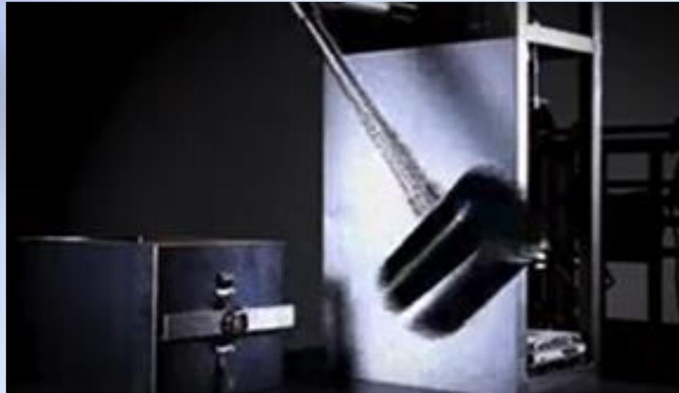
Figure 3. Example of a drop hammer for shock testing
